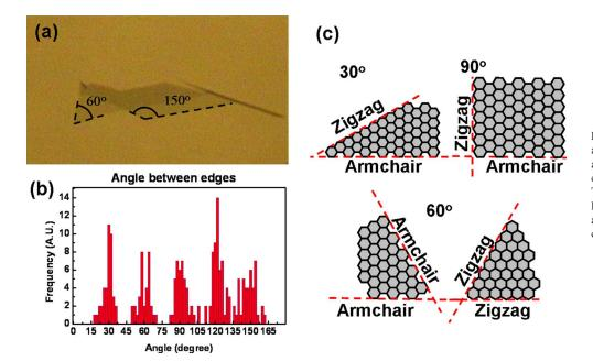
FIG. 1. (Color online) (a) Optical image of a typical MCG sheet and the angles between edges. (b) The statistical results of the angle measurements. The standard deviation is  $5.4^{\circ}$ . (c) Illustration of the relationship between angles and the chiralities of the adjacent edges.
